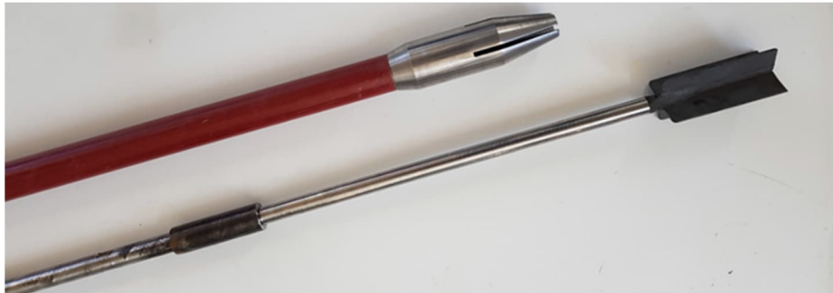
Figure 2. Upgraded “Geotek” field vane equipment of UX category with protective shoe and casing.
