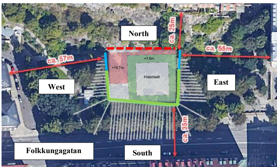
Figure 3 Lay-out of the secant pile wall (green) and soldier pile wall (blue), as well as the rock slope along the north side of the pit (red dotted line).
