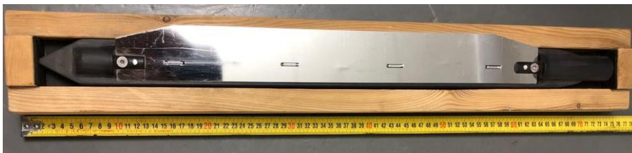
Figure 1 Peat Sampler with 40 mm diameter (also known as “Russian Corer”).
