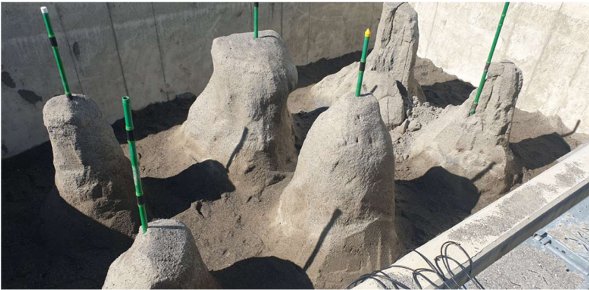
Figure 8. General view after exhuming biocemented sand columns
