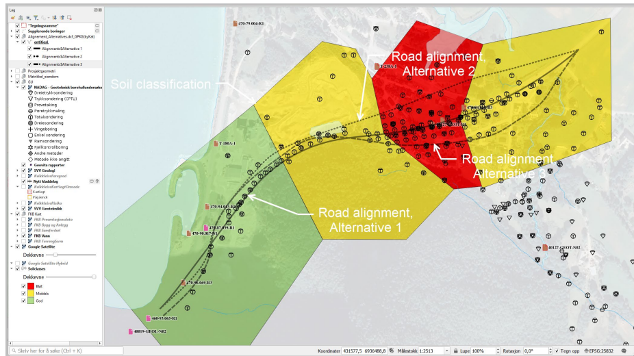
Figure 2 Areas defined by different soil classes together with road alignment alternatives in QGIS.
