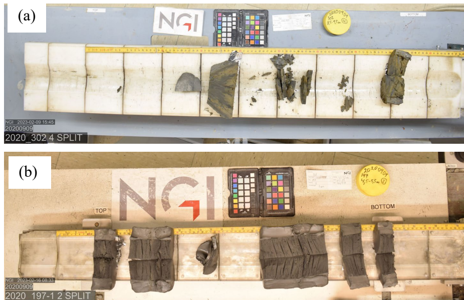
Figure 3. Piston samples. Examples of (a) dry crust intrusions, (b) laminated clay.
