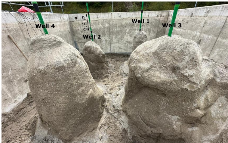
Figure 5, Sand columns obtained as a result of the MICP treatment applied in the upscaling experiment of Büyüklü et al. (2023) [7].
