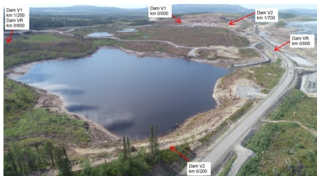
Figure 2. Drone photo over the dam area, to the right of the road you can see the construction of the dam V2 [12].
