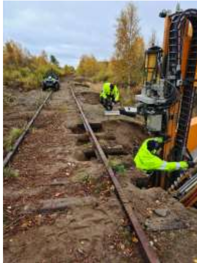
Figure 1 Investigations of peat at the (no longer used) railway at the test site Missenträsk.
